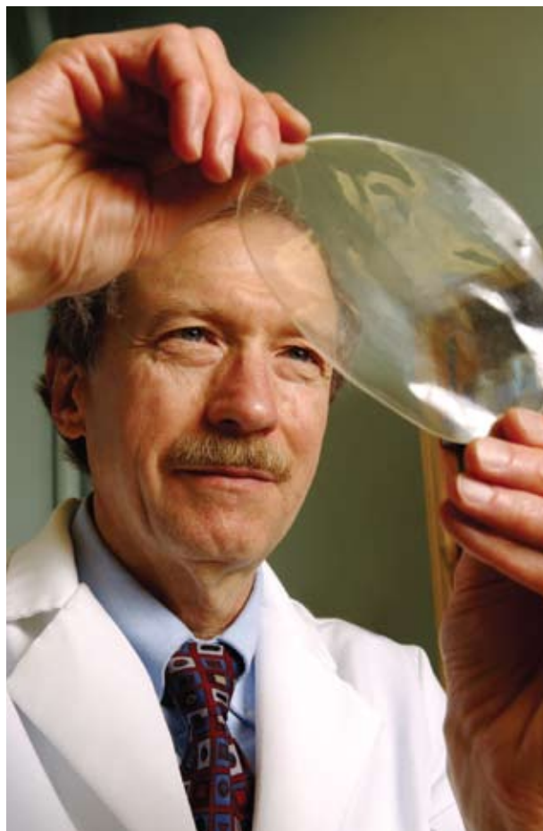
John Krochta, Professor of Food Science and Technology at the University of California, Davis, is shown holding up one of the whey protein films patented in 1996 for potential coating applications on nuts, dried foods, and fruits.
