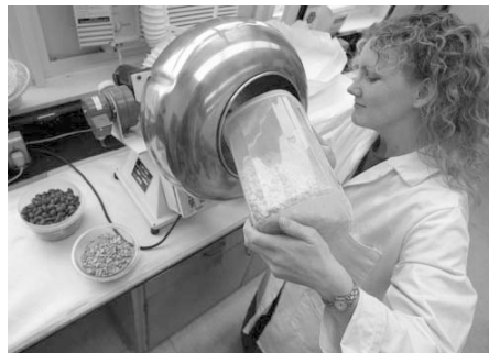
A UC Davis food science graduate student places peanuts into a pilot-scale confectioners pan for coating with a whey protein-based, oxygen-barrier coating formulation. The coating protects the peanuts from oxidative rancidity and thus extends shelf life of peanut-containing products.
