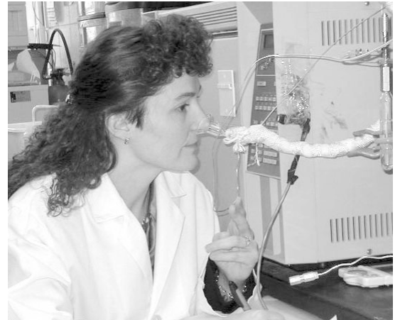
MaryAnne Drake, an associate professor of microbiology and sensory analysis at North Carolina State University, conducting gas chromatography olfactometry.
